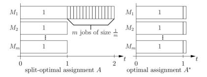
Figure 5.4: Worst-case example for split-optimal assignments.
